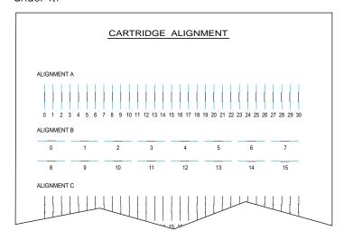
From each group on the test page, locate the number under the alignment pattern that comes closest to forming a perfectly straight line.
